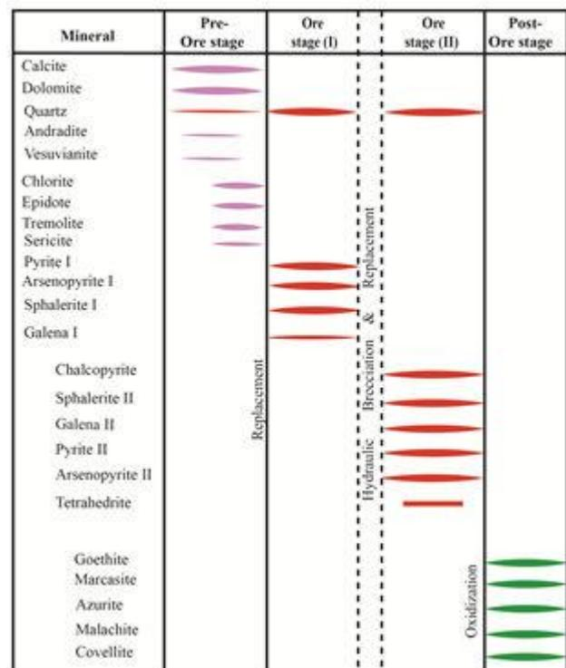
Figure 7) Simplified paragenetic sequence of the assemblages of main ore in the Amensif deposit.
