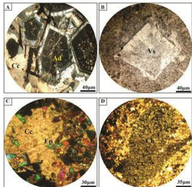
Figure 6) (A) Photomicrograph of subhedral andradite crystal showing concentric-oscillating zoning. (B) Photomicrograph of prismatic phenocrystal of vesuvianite. (C and D) Photomicrographs showing replacement between calcite/ dolomite and epidote and or chlorite Mineral abbreviations: Dl-dolomite; Cc-calcite; Ep-epidote; Ad-andradite; Vs-vesuvianite.
