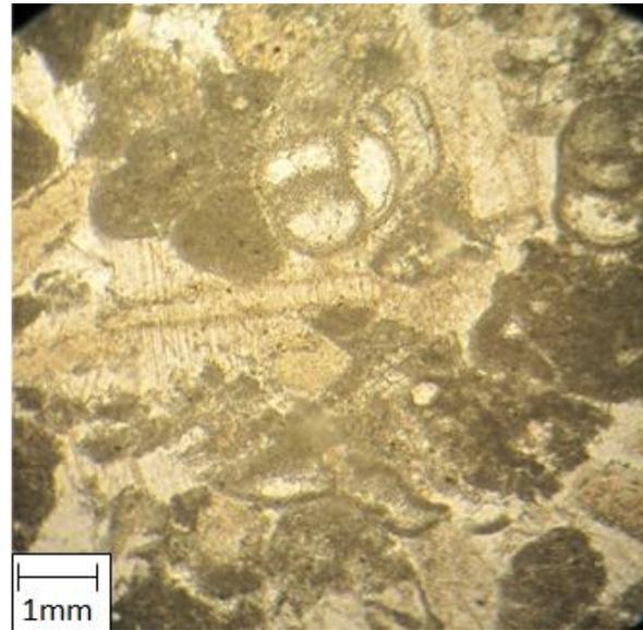
Figure 10) Microphotograph of bioclast intraclast packstone facies belt lagoon.
