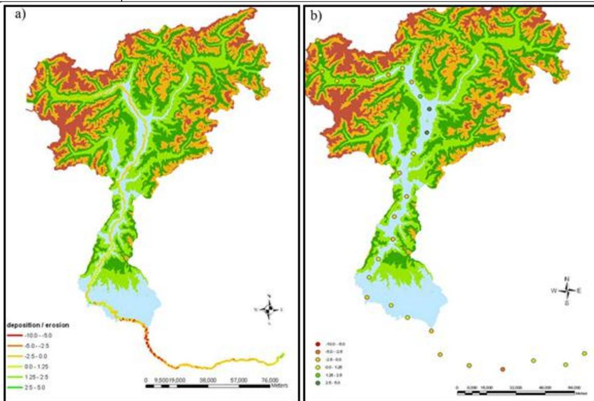
Figure 2) Evolution of the Adige River between 1954 and 1996: a) measured values, b) computed values.
