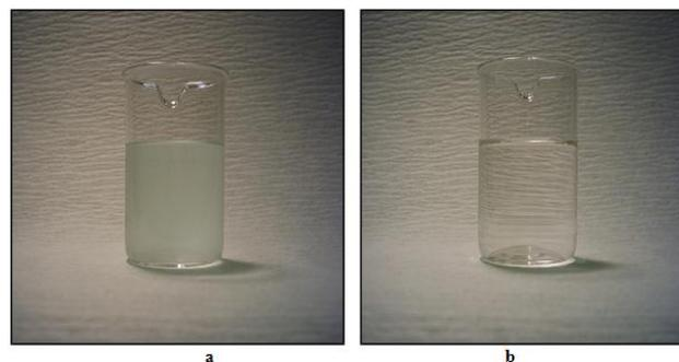
Figure 3) Comparison of DNPDSSE method raffinates: a) before precipitate flotation and b) after precipitate flotation.
