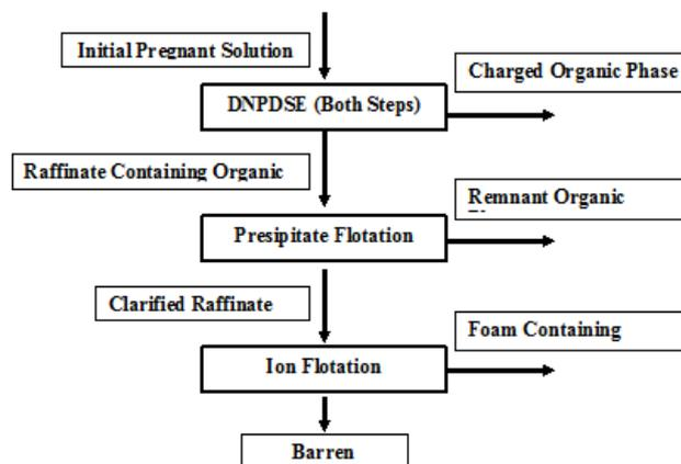
Figure 4) Flow sheet of the DNPDSSE-PF-IF methods.
