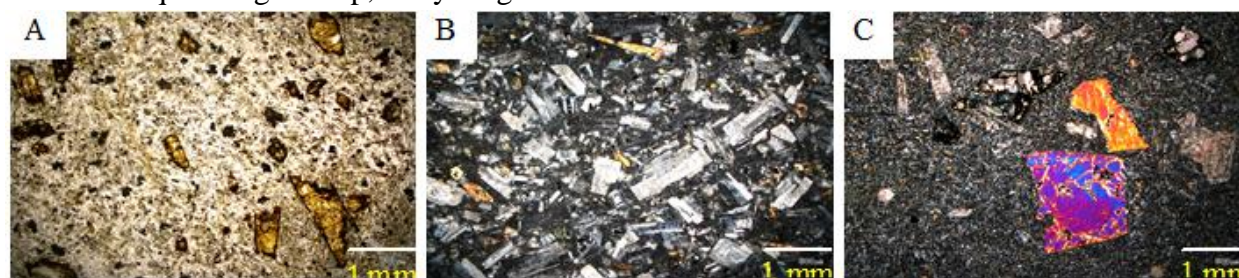
Figure 4) Microscopic images of rock samples: A - andesite - amphibole of the opacities, B-diorite porphyry, C-andesite basalt - the presence of olivine and pyroxene as phenocrysts in the background of Plagioclase microlite XPL.
